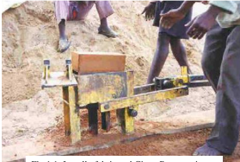
Fig 1.1: Locally fabricated Cinva Ram on site
