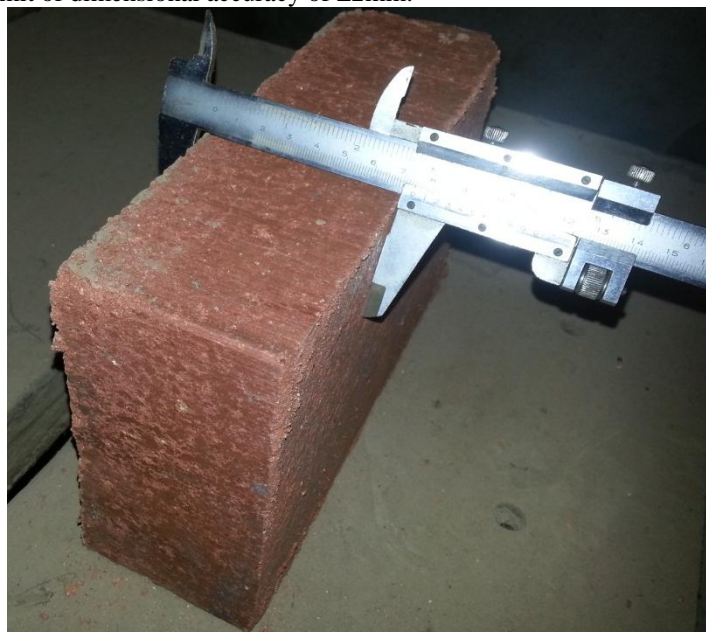
Figure 3.3 Dry Block being measured with Vanier Calipers
