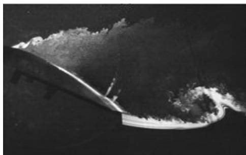
Fig 10: snap short of smoke flow visualization after 12 degree AOA.
