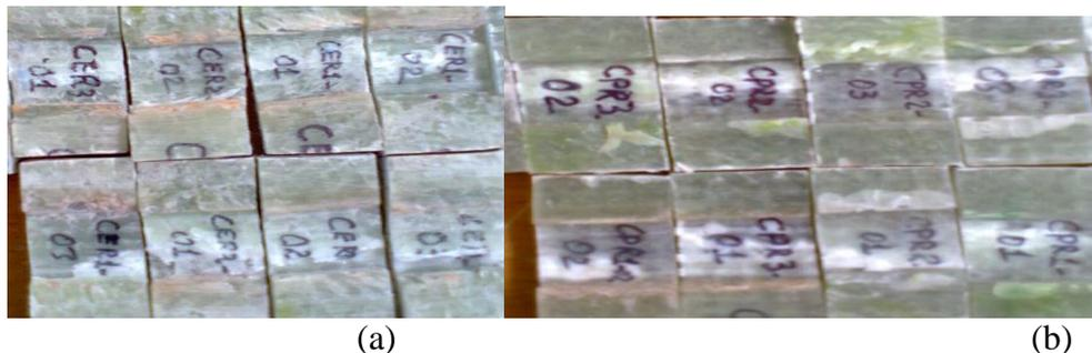
Fig. 11 Compressive failure modes (a) E-glass/Epoxy and (b) E-glass/Polyester composites
