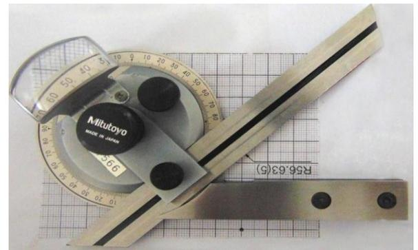
figure 10-Measurement of spring back using bevel protractor
