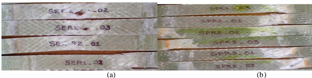
Fig. 9 In-plane Shear Failure modes (a) E-glass/Epoxy composite (b) E-glass/Polyester Composite
