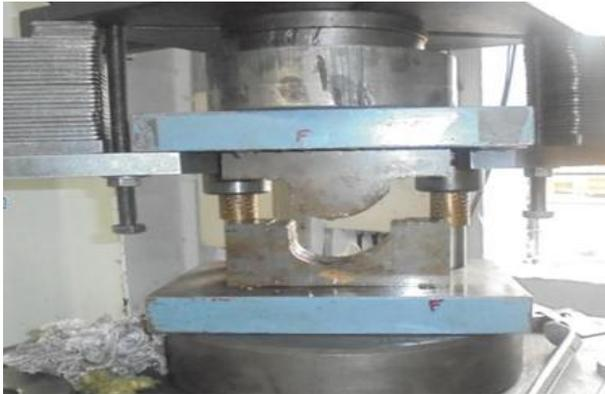
figure 7:Die Fixed in hydraulic press
