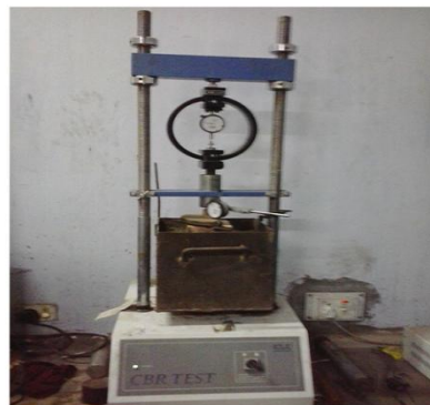
Fig. 2 General arrangement and loading the sample
