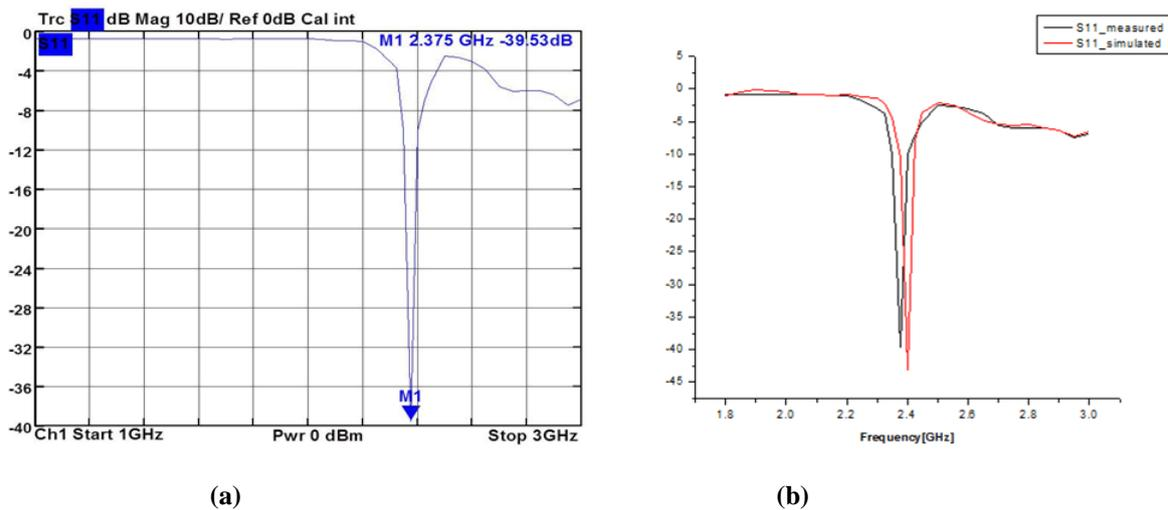
Figure 8. (a) VNA Screen Output (b) Compared measured and simulated results
