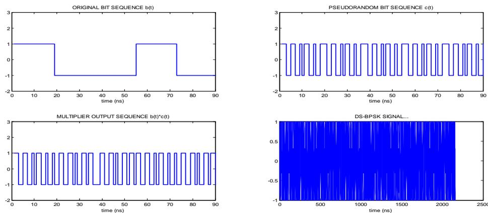
Figure 12. Waveforms for the digital communication system
