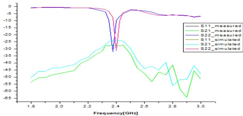
Figure 10. Comparison results for simulated and measured for 2X2 MIMO System
