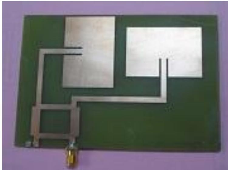
Figure 7. Photograph of fabricated antenna
