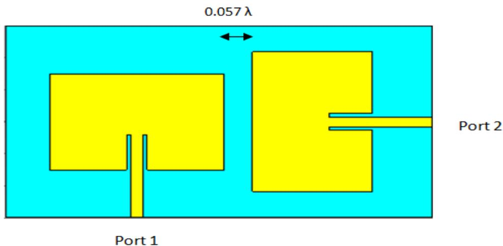
Figure 3. MIMO antenna array having two ports
