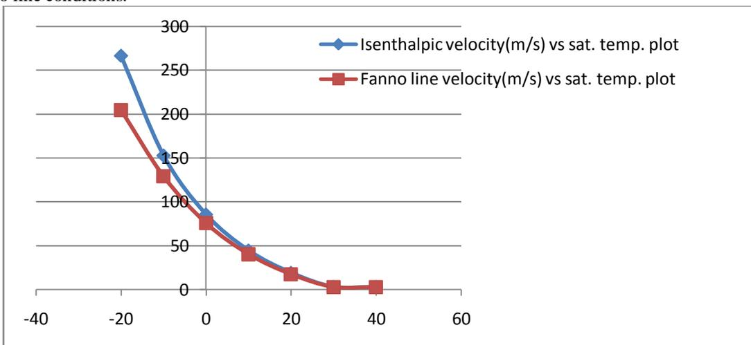
Fig-3. Isenthalpic and actual Fanno line velocity VS saturation temperature plot for refrigerant in the capillary.
