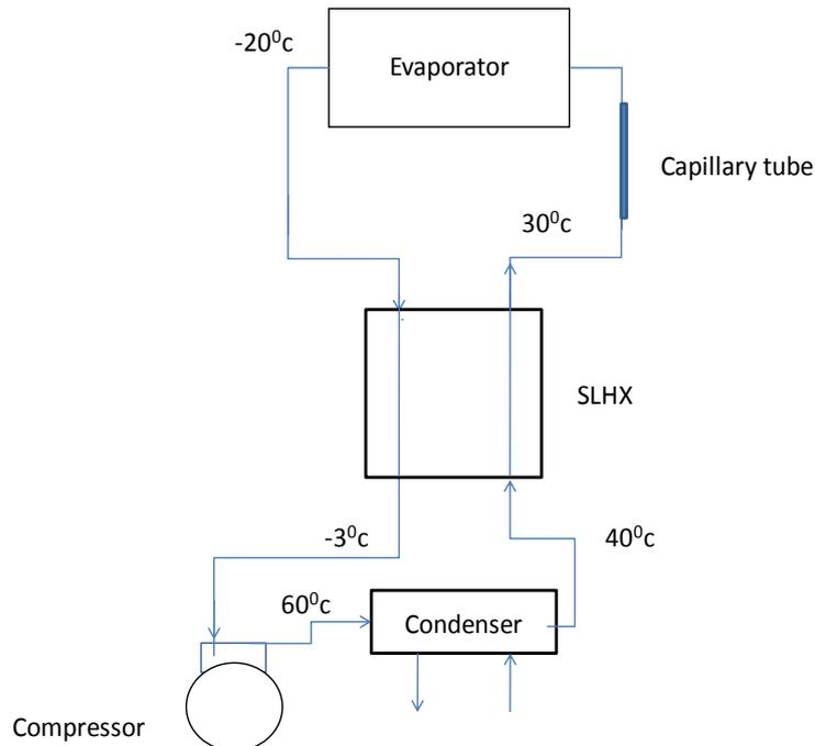
**Fig-1. Positions of installation of non adiabatic SLHX & adiabatic capillary tube in VCRS.**
