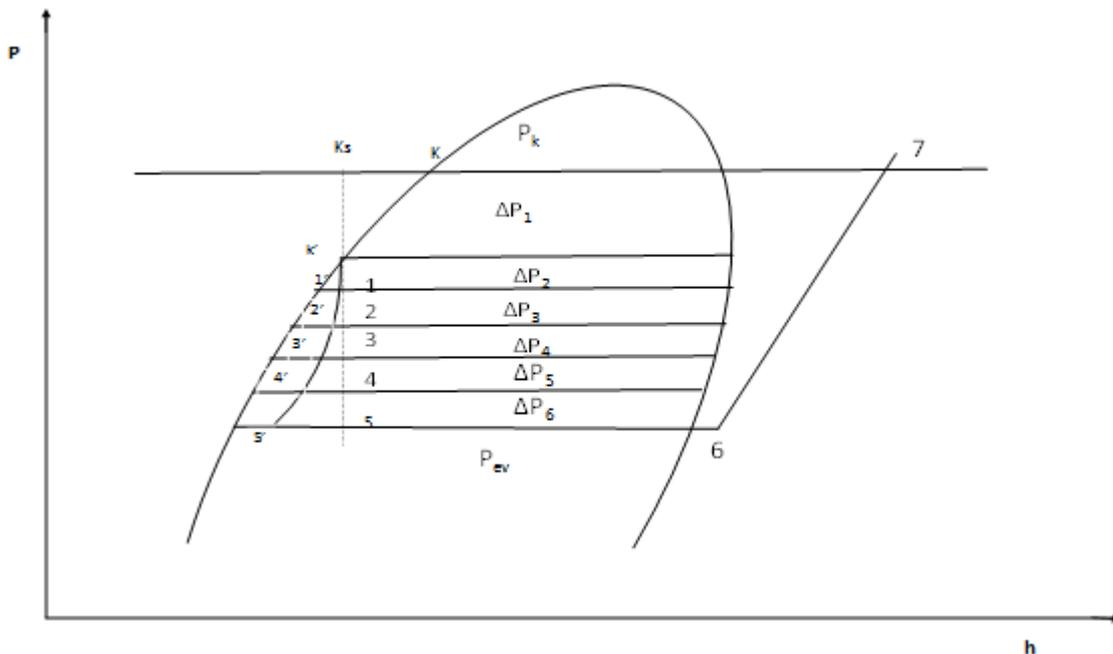
Fig-2. Ph Chart for Pressure & enthalpy changes of elementary lengths of the capillary along Isenthalpic and Fanno line considering sub cooling of condensate by SLHX.
