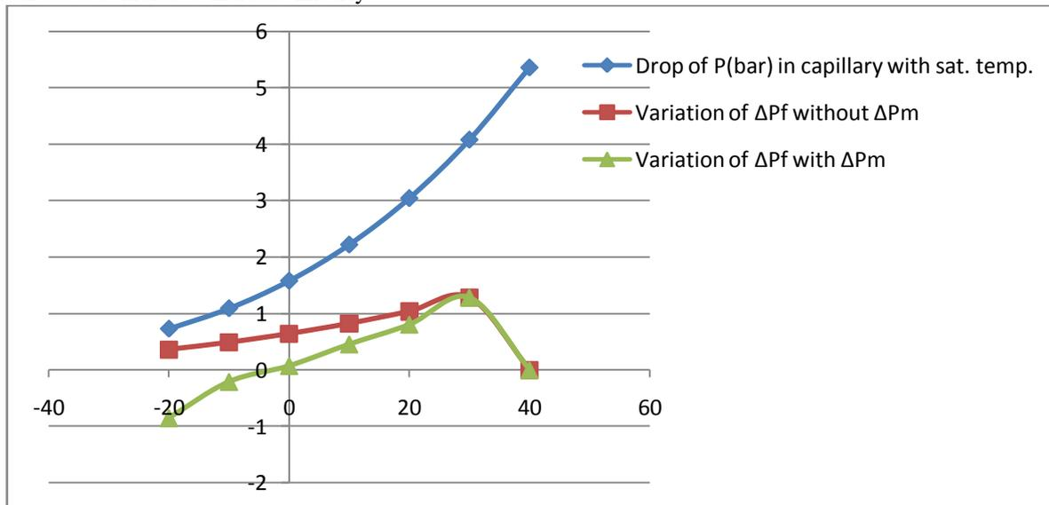
Fig-4. Actual pressure (bar) variation & elementary frictional pressure drop considering with and without momentum gain vs saturation temperature (<sup>o</sup>c) drop plots.
