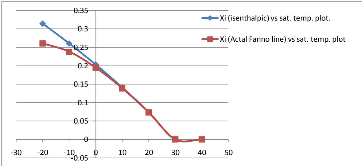
Fig-3. Isenthalpic and actual Fanno line refrigerant quality VS saturation temperature plot for refrigerant in the capillary.
