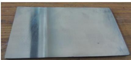
Fig 4.2 Substrate after grinding
