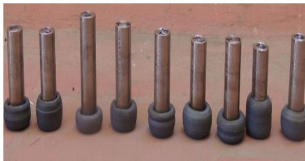
Fig 4.4 Length of mechatrodre after friction surfacing
