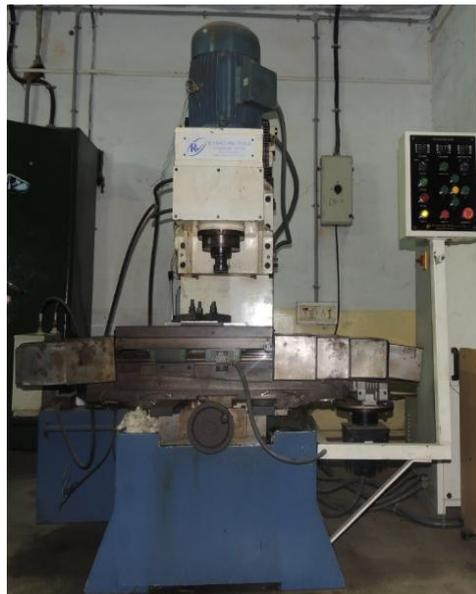
Fig 4.3 Experimental setup of friction surfacing machine
