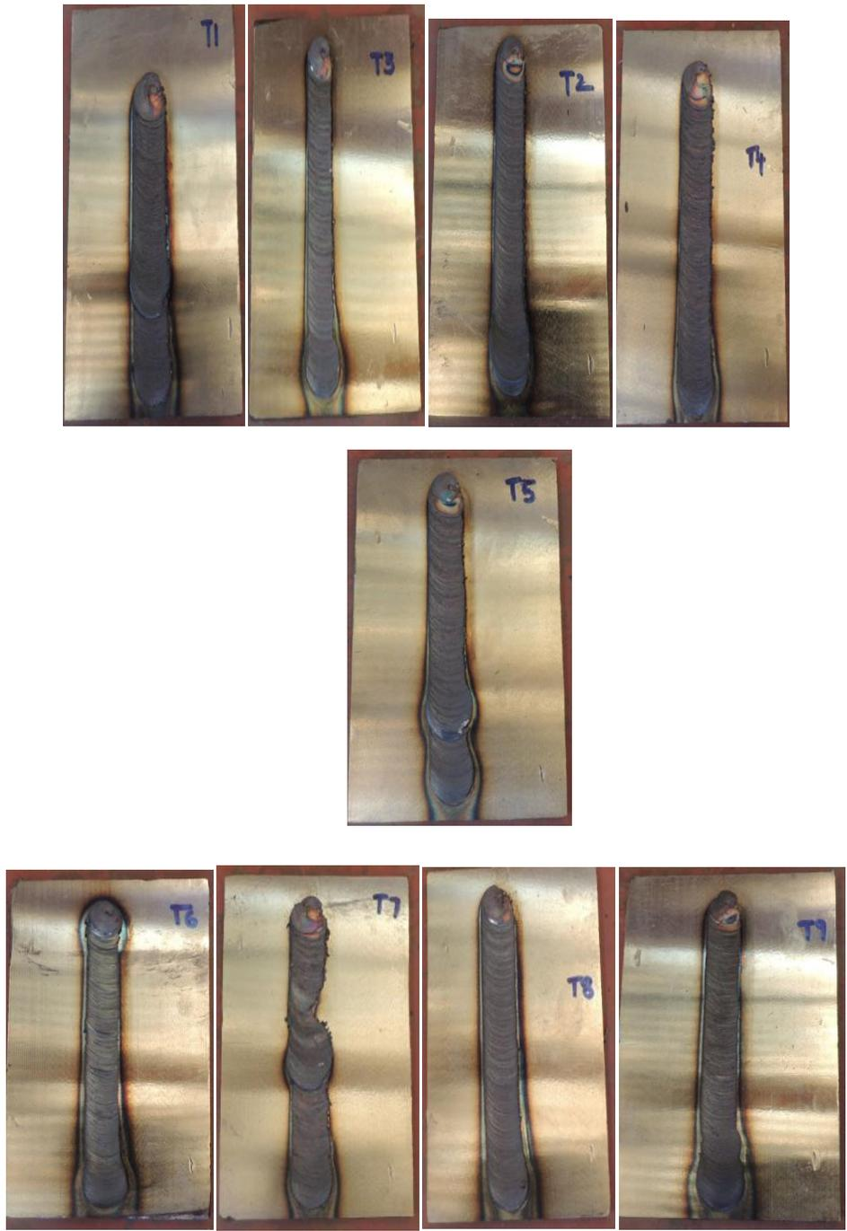
4.7.1 Coating Thickness ( $C_t$ ) on Deposit Geometry
