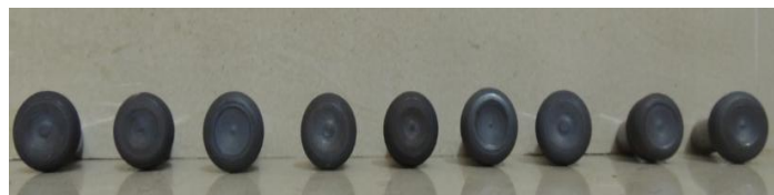
Fig 4.5 Diameter of mechatrode after friction surfacing
