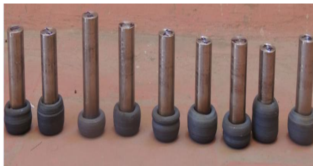
Fig 4.4 Length of mechatrodre after friction surfacing
