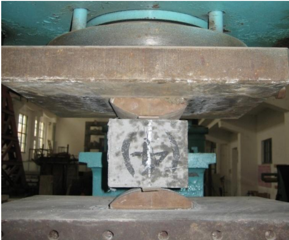
Fig. 2. Test set-up for splitting tensile strength
