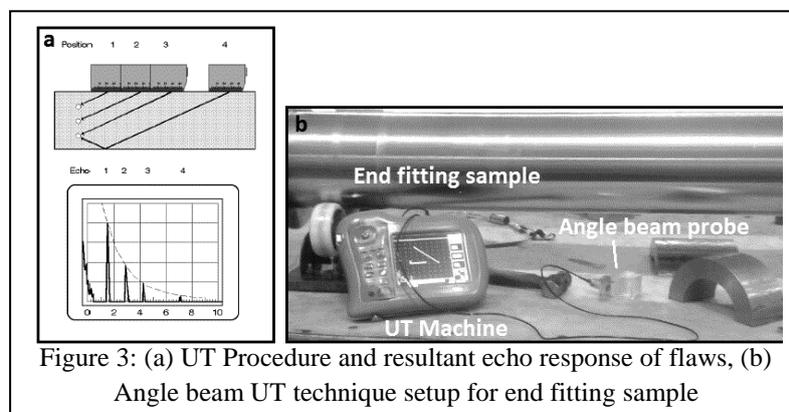
Figure 3: (a) UT Procedure and resultant echo response of flaws, (b) Angle beam UT technique setup for end fitting sample
