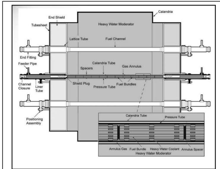
Figure 2: Basic schematic of CANDU reactor core components
