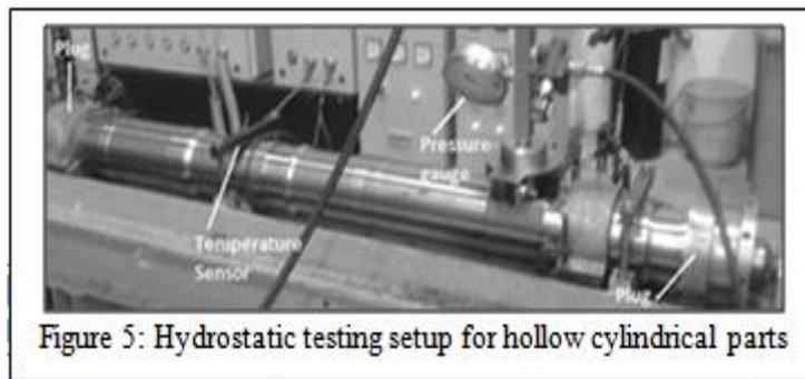
Figure 5: Hydrostatic testing setup for hollow cylindrical parts
