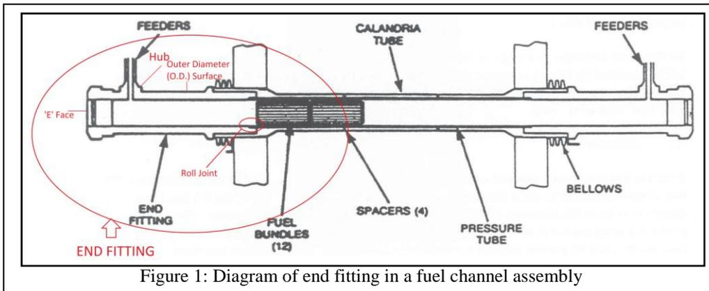
Figure 1: Diagram of end fitting in a fuel channel assembly
