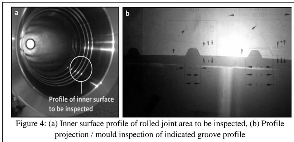
Figure 4: (a) Inner surface profile of rolled joint area to be inspected, (b) Profile projection / mould inspection of indicated groove profile
