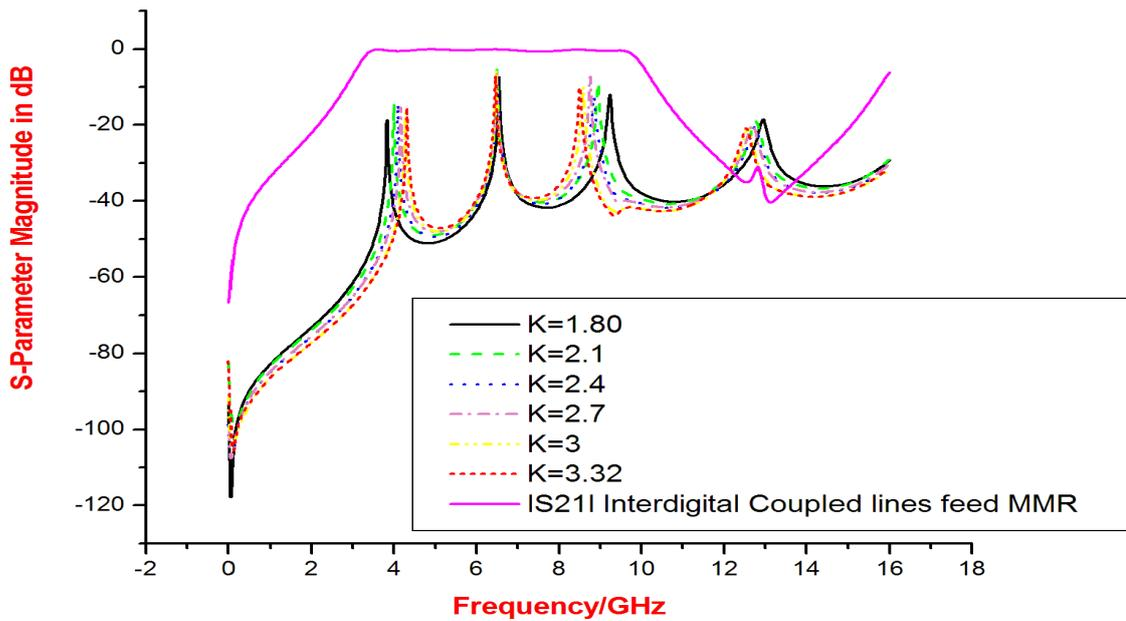
Fig. 4 Comparison of simulated detuned resonant frequencies with variation in impedance ratio (a) K=1.80 (b) K=2.1 (c) K=2.4 (d) K=2.7 (e) K=3 (f) K=3.32 and  $S_{21}$ [dB] of tuned MMR feed by interdigital coupled lines
