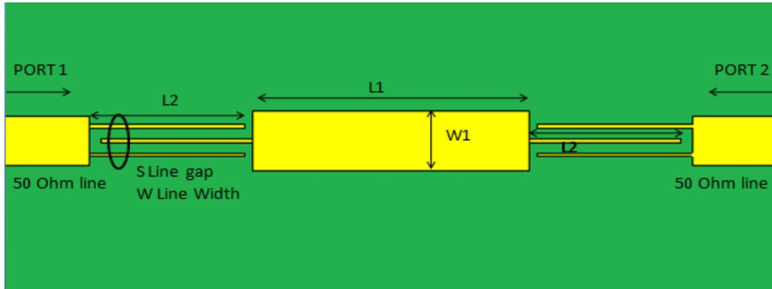
Fig 1. Layout of the proposed UWB bandpass filter
