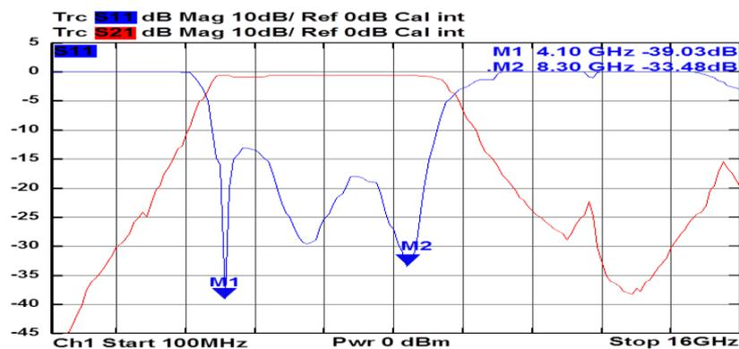
Fig. 8 Fabricated measured result of proposed UWB BPF
