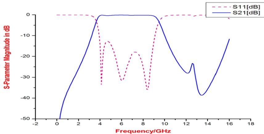
Fig. 7 Simulated result of proposed UWB BPF
