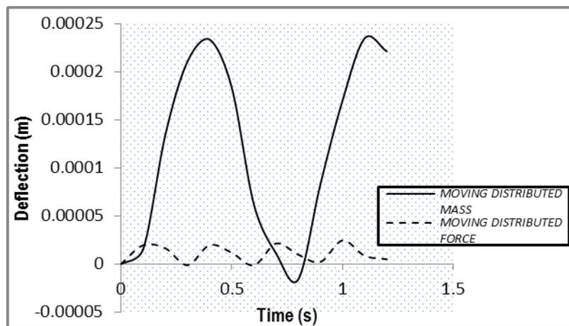
**Fig.7:** Comparison of the displacement response of simply supported Bernoulli-Euler beam resting on bi-parametric elastic foundation for fixed values of foundation stiffness, axial force and shear modulus.
