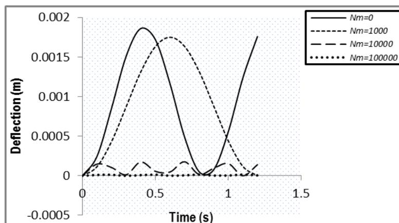
**Fig.2:** Displacement response of simply supported Bernoulli-Euler beam for moving distributed mass for various values of axial force  $N_m$  and fixed values of shear modulus and foundation stiffness.
