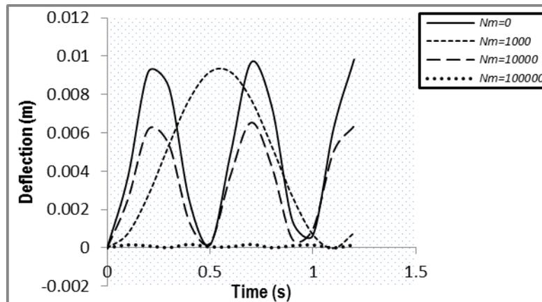
**Fig.1:** Displacement response of simply supported Bernoulli-Euler beam for moving distributed force for various values of axial force  $N_m$  and fixed values of shear modulus and foundation stiffness.
