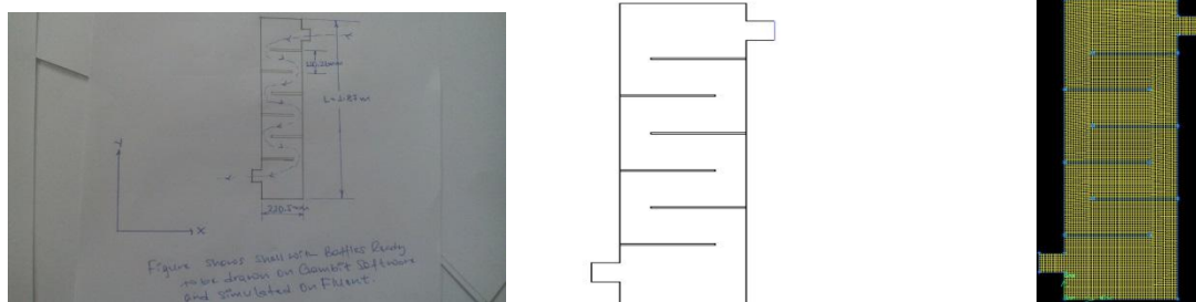
Figure8. a).STHEx drawn by hand b).STHEx drawn on Gambit c). STHEX Meshed on Gambit
