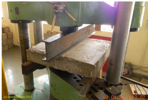
Figure 1: BRC slab under test
