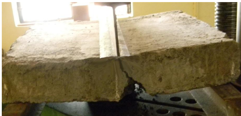
Figure 3: BRC slab failure
