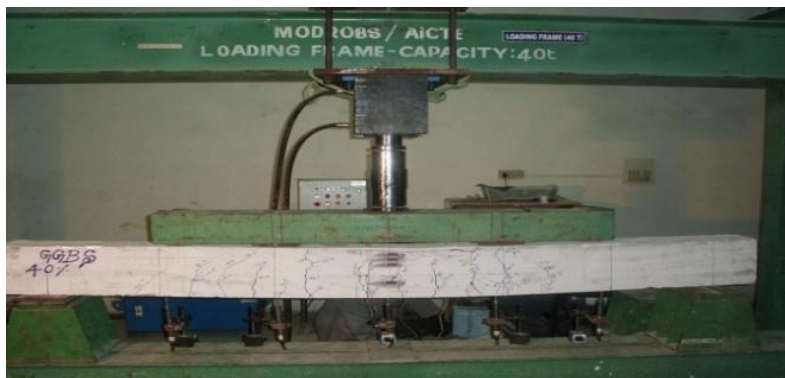
Fig. 3: Failure Pattern of the beams with 40% GGBS
