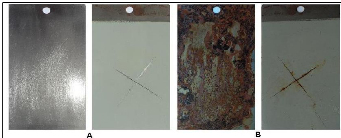
Figure 4– Development of the corrosion process (three days).
