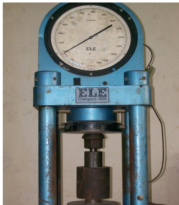
Fig. 1: Extrusion setup on ELE Compact-1500 hydraulic machine
