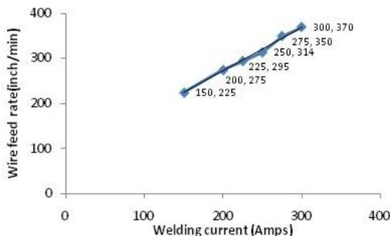
Fig. 2. Relationship between Current and Wire Feed Rate
