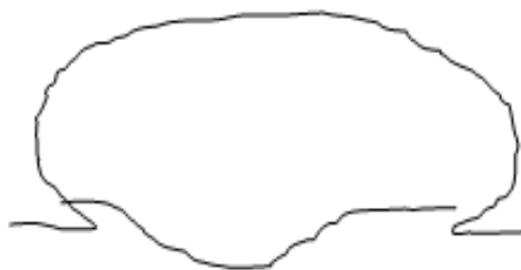
Fig. 3. Traced Profile of bead geometry
