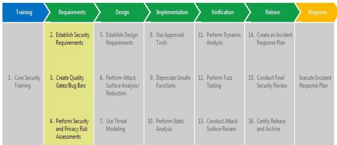
Fig 1. security development lifecycle: requirements phase
