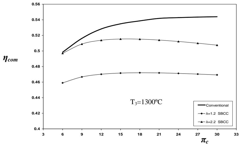
Fig. 9: Comparison between the efficiency of SBCC and conventional combined cycles.
