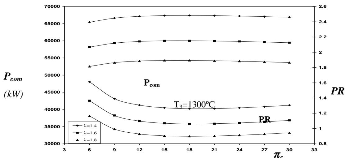
**Fig. 2: The SBCC output power and power ratio at fixed T<sub>3</sub> of 1300°C and at three different excess air factors.**
