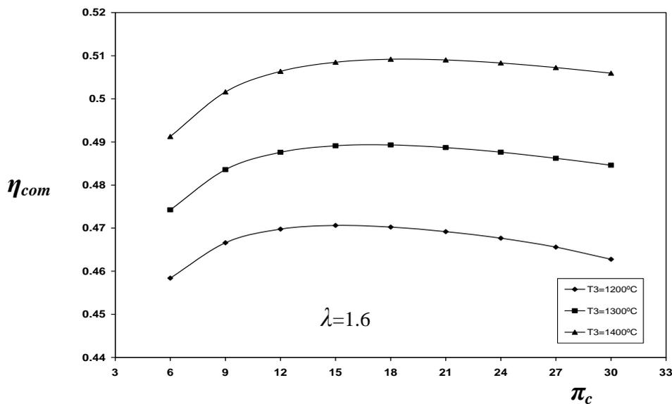
Fig. 7: Thermal performance of the SBCC at different turbine inlet temperatures.
