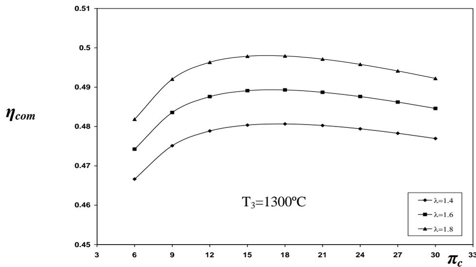
Fig. 3: The SBCC energy efficiency at fixed T<sub>3</sub> of 1300°C and at three different excess air factors.
