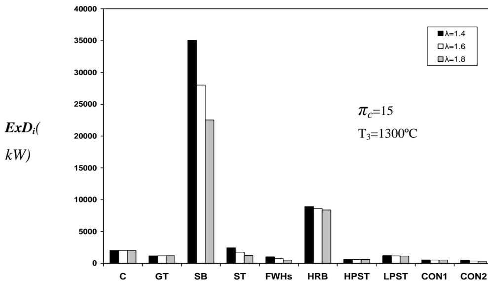
Fig. 5: Exergy destructions in the cycle components at different excess air factors.
