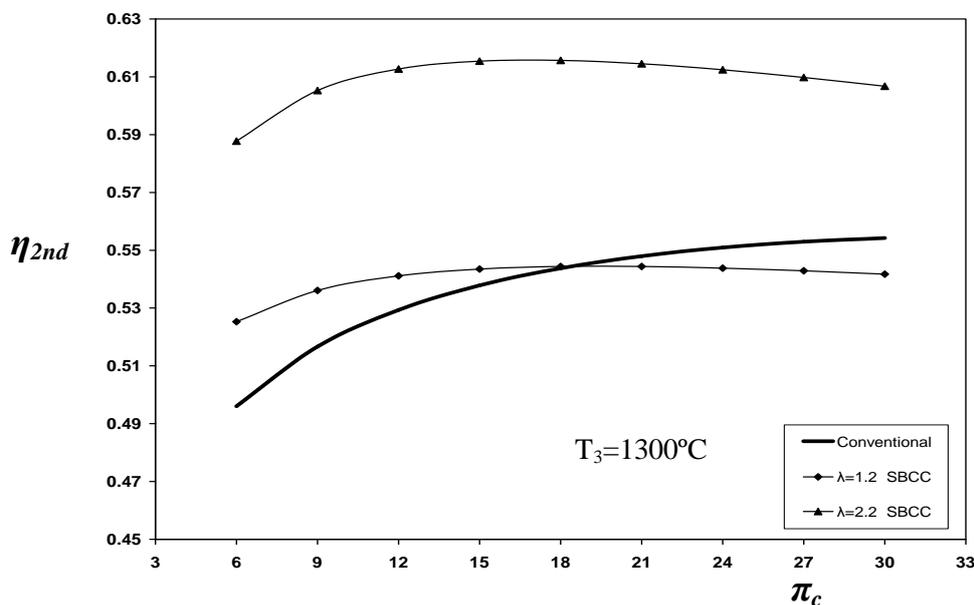
Fig. 10: Comparison between the second-law efficiency for SBCC and conventional combined cycles.
