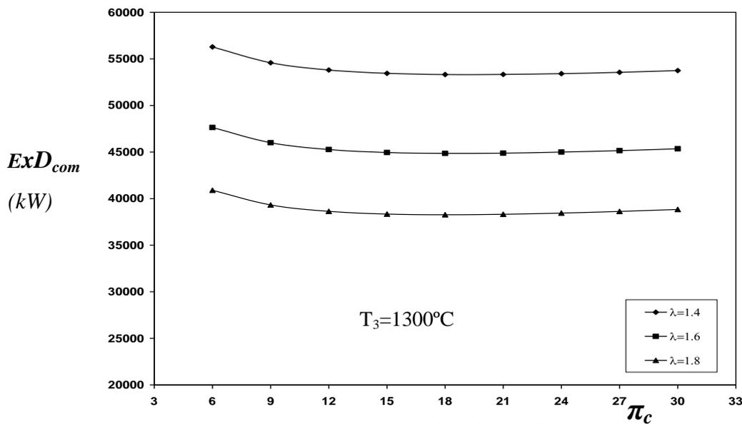
Fig. 4: Total exergy destruction in the SBCC at different excess air factors.
