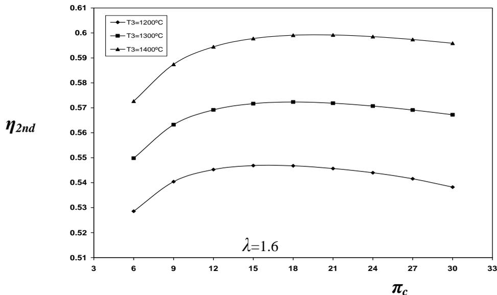
Fig. 8: The second-law efficiency of the SBCC at different turbine inlet temperatures.
