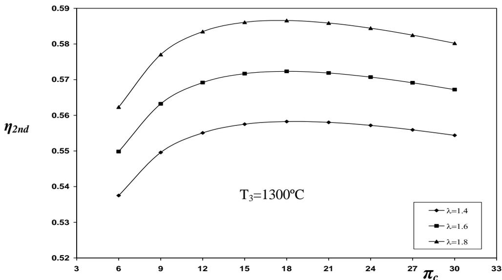
Fig. 6: Second-law efficiency of the SBCC at different excess air factors.
