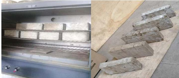
Figure 3. The Brick Visibility Test in Oven-Dry Condition
