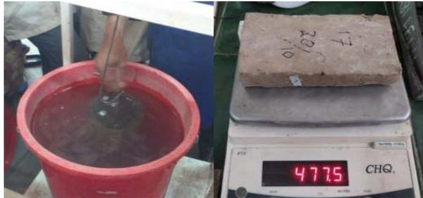
Figure 7. The Brick Apparent Density Test
