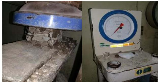
**Figure 5.** The Bricks Compressive Strength Test**Table 7.** The Bricks Compressive Strength Test Results
