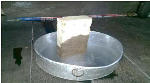
Figure 6. Soaking Bricks for Salt Crystals Observation
