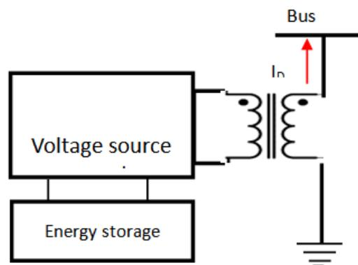
Figure 1. D-STATCOM model
