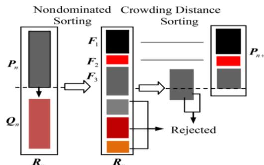
Figure 3. NSGA-II procedure
