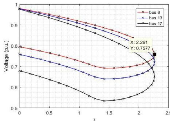
**Figure 9. PV-curve with D-STATCOM**
