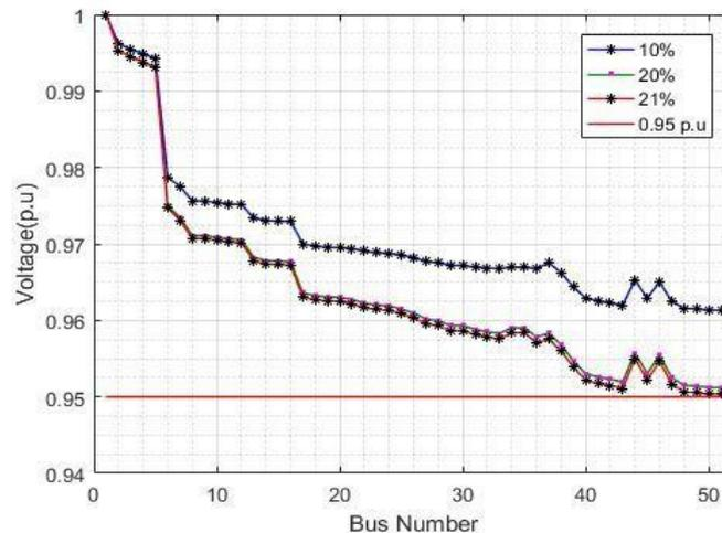
Figure 10. Voltage profile with different load factor
