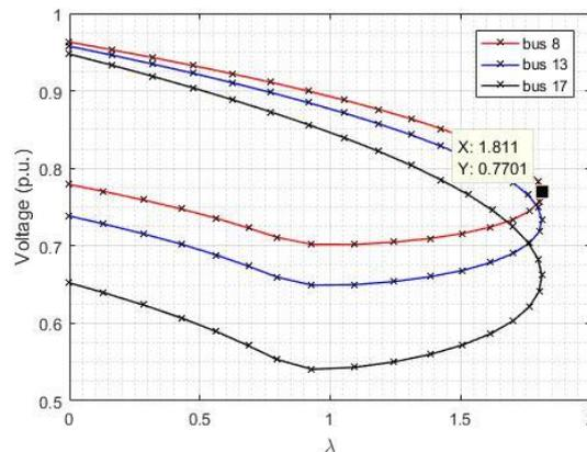
**Figure 8. PV-curve without D-STATCOM**
