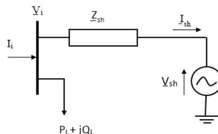
Figure 2. Simplified model of D-STATCO
