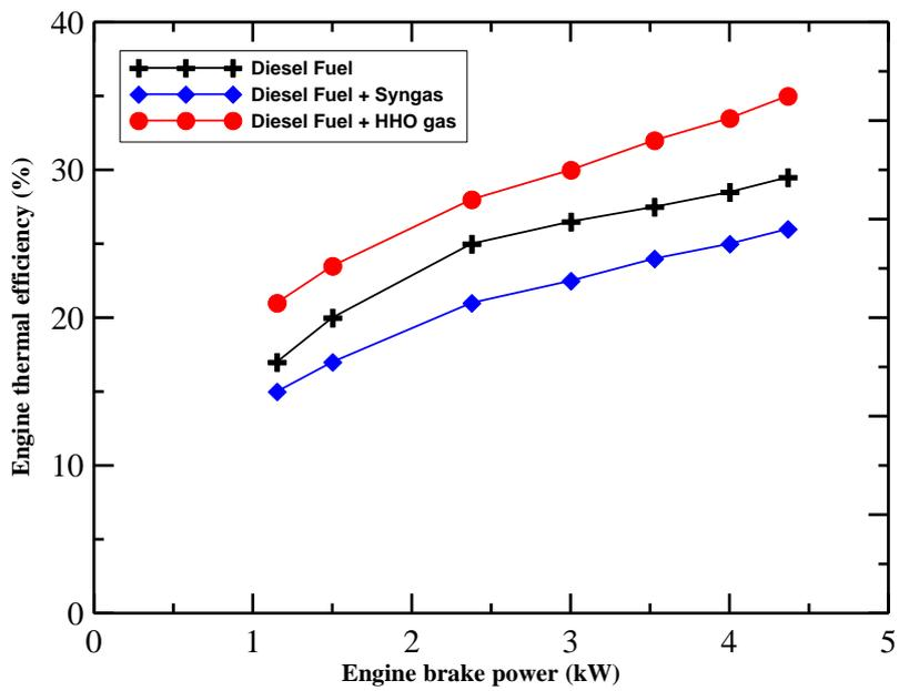
Fig. (5): The variation of engine thermal efficiency with brake power
