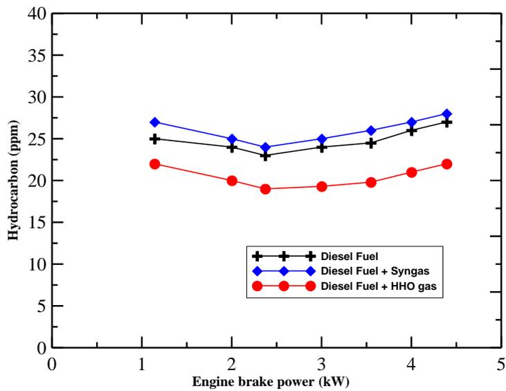
Fig. (9): The variation of HC emission with engine brake power
