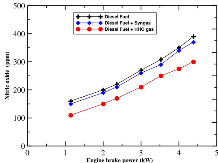
Fig. (10): The variation of NO emission with engine brake power
