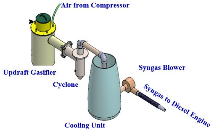
Fig. (2): Schematic diagram of the gasification plant.
