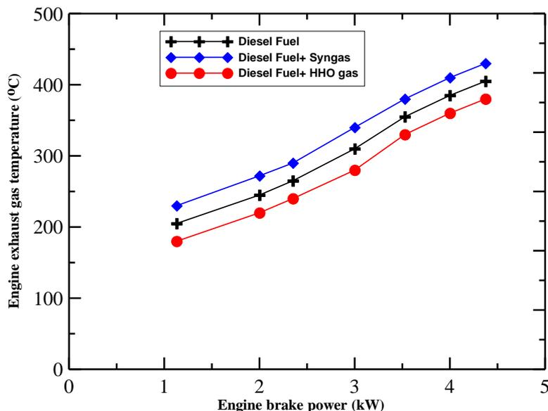
Fig. (7): The variation of engine exhaust gas temperature with brake power
