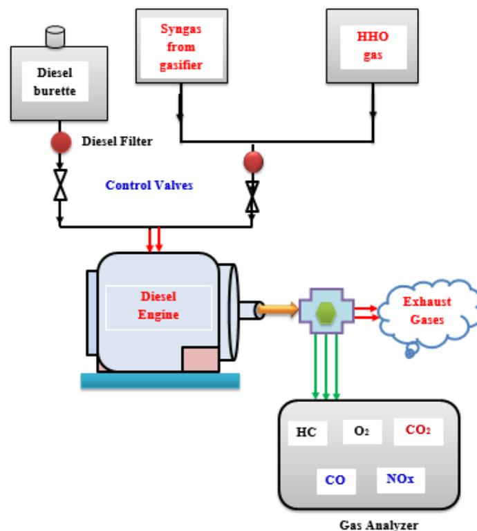
Fig. (1): Schematic diagram of the experimental setup.
