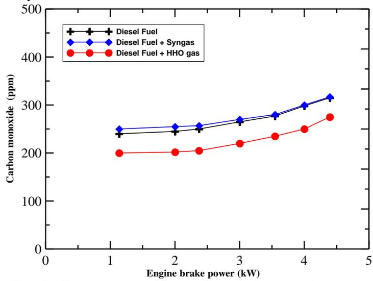
Fig. (8): The variation of CO emission with engine brake power.
