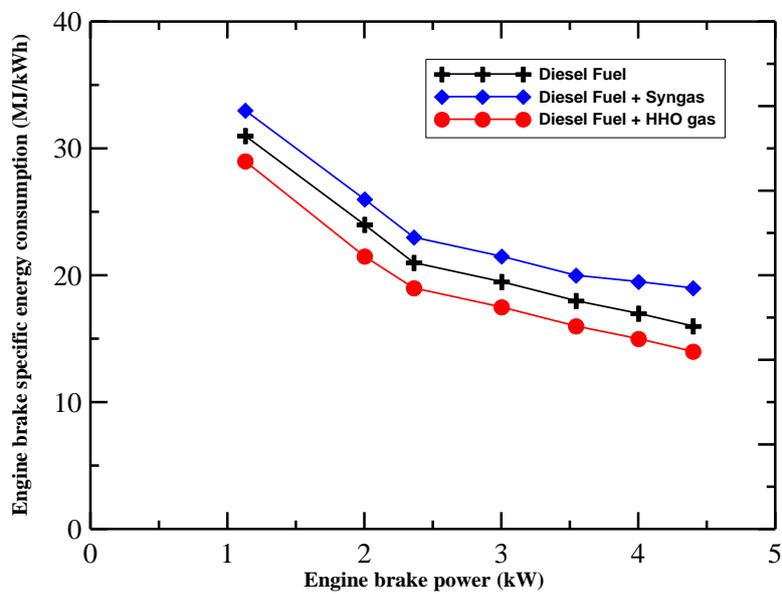
Fig. (6): The variation of engine brake specific energy consumption with brake power
