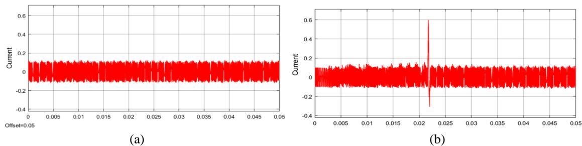
**Fig. 9. d-axis current for (a) pre fault condition and (b) pre fault to post fault condition.**
