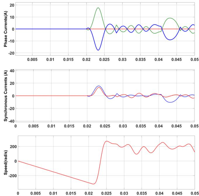
Fig. 7. Simulation results showing phase currents, synchronous currents and speed for post fault.
