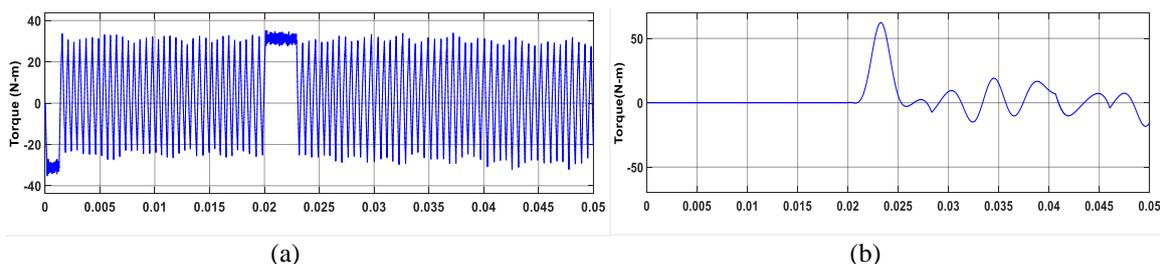
Fig. 8. Electromagnetic Torque for (a) pre fault condition and (b) post fault condition.
