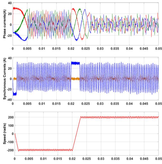
Fig. 6. Simulation results showing phase currents, synchronous currents and speed for pre fault.
