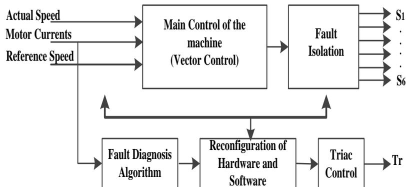
Fig. 3. Block diagram of the fault tolerant control system.
