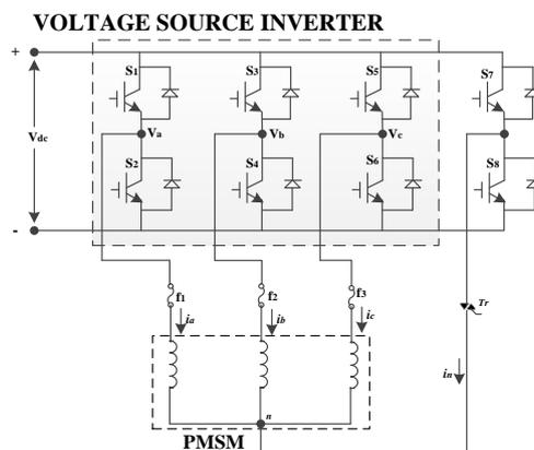
Fig. 2. Fault Tolerant PMSM Drive.
