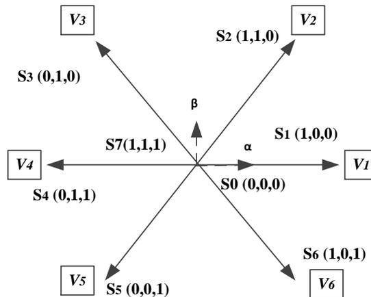
**Fig. 4. Voltage vectors and corresponding switching states of the inverter.**
