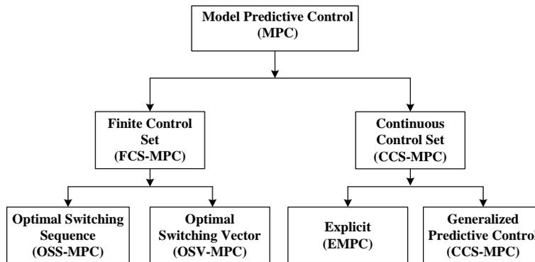
Fig. 1. MPC strategies applied to power converter and drives.
