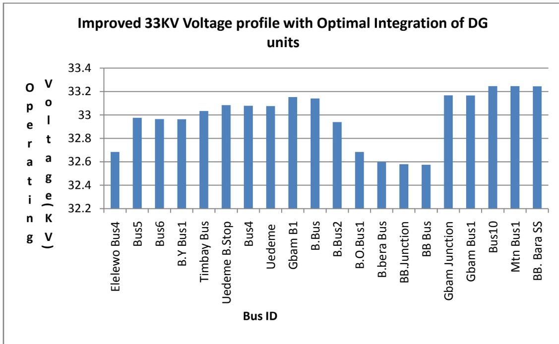
Fig.4.2 shows the voltage profile improvement on 33KV, from Elelewo Bus4-BB.Barra SS. respectively, representing the voltage profile with optimal placement of the distributed generation units. The chart shows the bus identities with their respective improved voltage, as seen from the chart a very good improvement was achieved from the 23.14KV Gbam B1 least voltage of 33KV base case (table 4.2) to 33.14KV on B.Bus located at Bunu Tai community.
