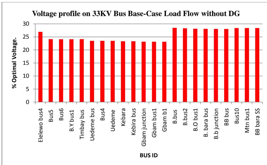
**Fig 4.1** above shows the voltage profile on 33KV bus base case load flow without the placement of distributed generation, from Elelewo bus4 – BB bara SS. As seen from the fig. The busses are accompanied with
