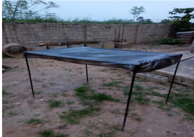
Figure 3: Dew water collection platform
