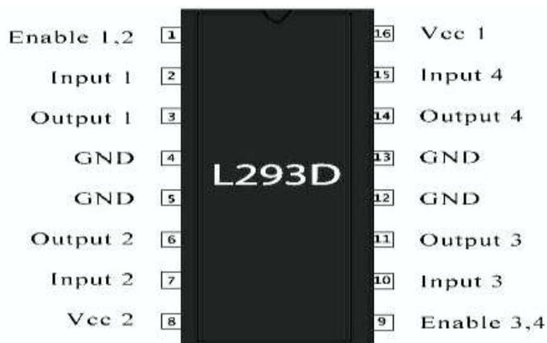
Figure 3: Pin diagram of L293D
