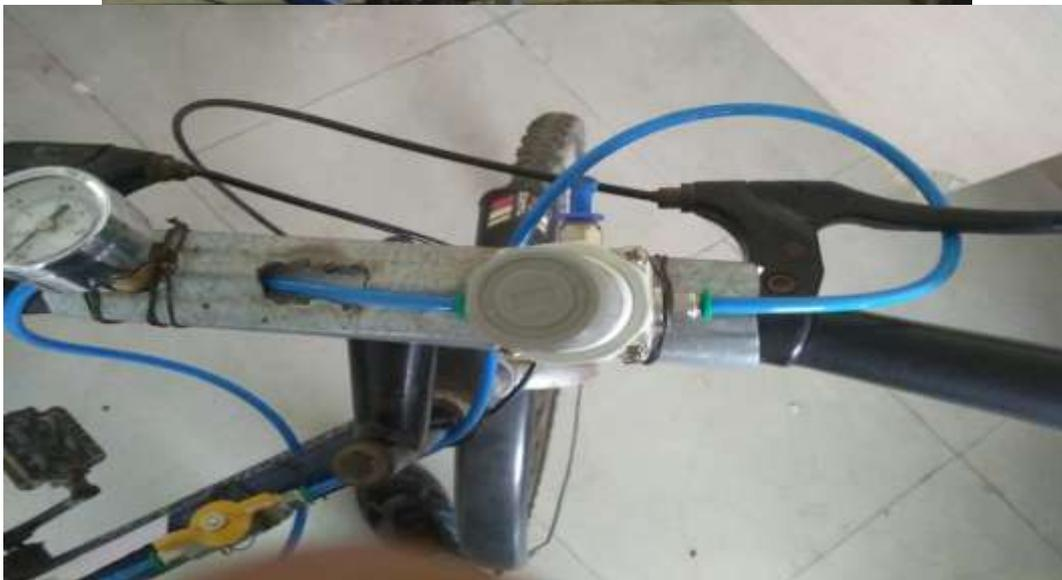
**3.5 DESIGN METHODOLOGY:** Welding an offset to the main rear support of wheel to hold the crank. A secondary free wheel welded to normal market supply. Created clip using galvanized tin at workshop. An auxiliary supported is cut out of tin sheet and bolted to main handle with all the mountings. A light weight mild steel disc was used initially which later replaced with a light aluminum disc due to buckling. It sufficiently reduced the inertia of part during very start of pedaling.
