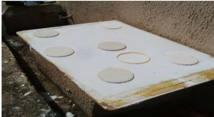
Plate 1: Curing of Moulded POP-RHA samples.
