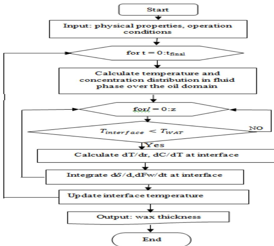
Figure 2.2: Program flowchart for amount of wax deposition
