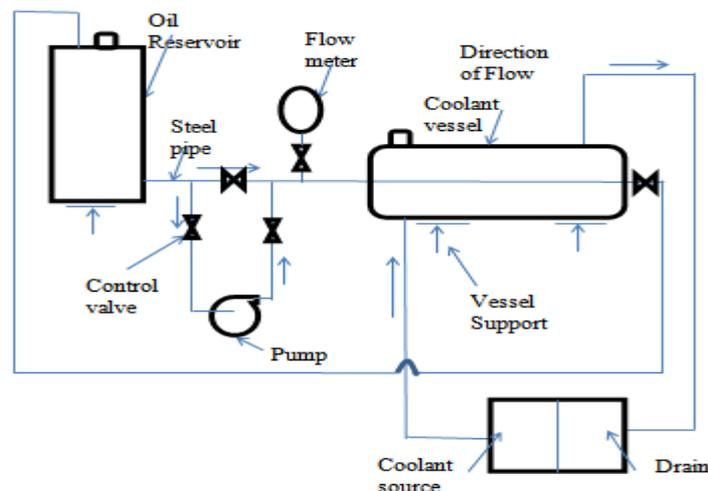
Figure 2.3: Schematic diagram of Laboratory Flow Loop
