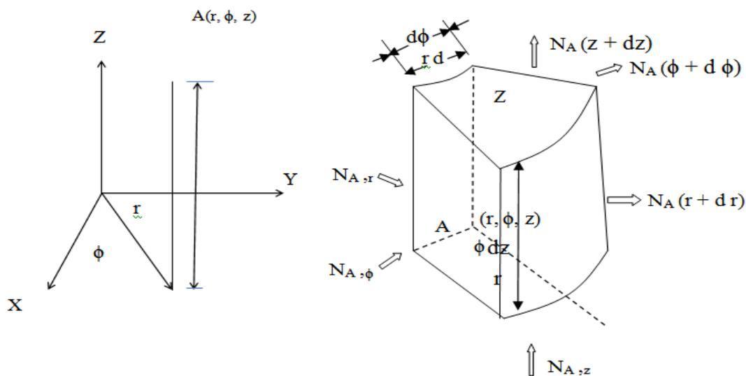
**Figure 1 Elemental volumes for three dimensional mass transfer analysis- cylindrical co-ordinates**
