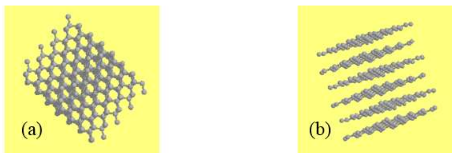
Figure 1. (a) Diamond structure and (b) graphite's layered structure [12].
