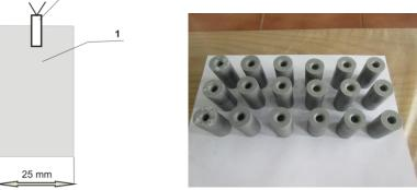
Fig. 2.Schematic and photo of the investigated pressed charges: 1 - composite, 2 -detonator
