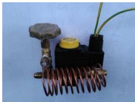
Figure 5. Solenoid valve and the capillary tube, as the LPG fuel flow regulator
