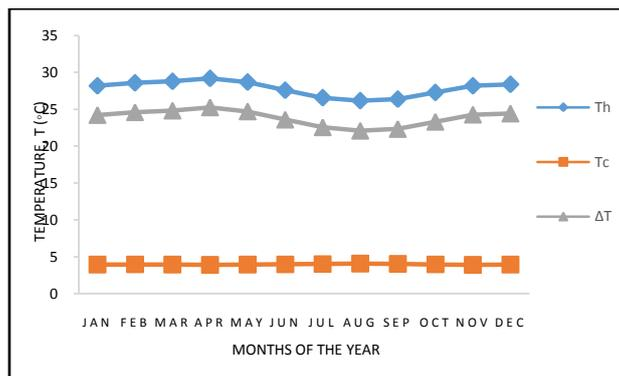
**Figure 5 :** Variation in Monthly Average Temperatures of Sea Surface Water,  $T_h$ , that at 1000m Depth,  $T_c$ , and the Difference  $\Delta T$ .
