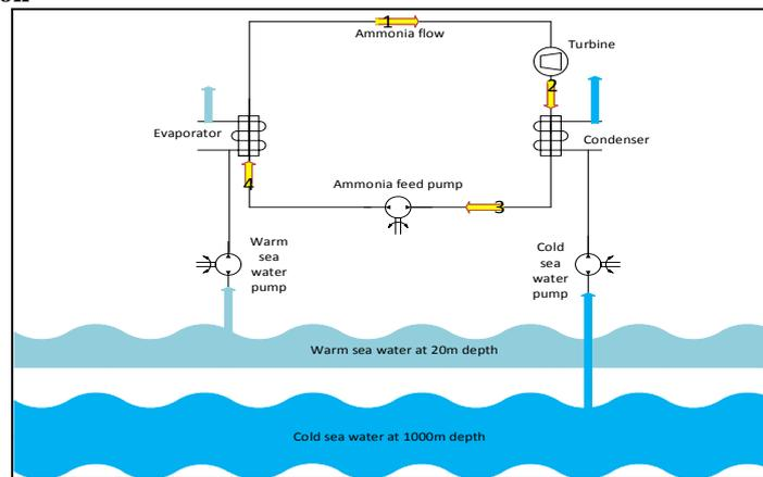
Figure 3: Schematic Diagram of the Close-Cycle OTEC Plant.
