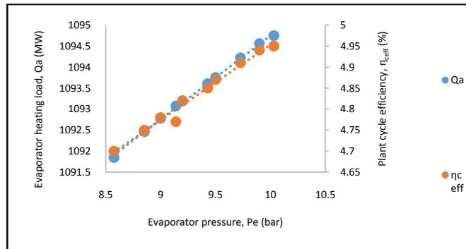
**Figure 7:** Variation of Evaporator Heating Load,  $Q_a$ , Plant Cycle Efficiency,  $\eta_{c\_eff}$  with Evaporator Pressure,  $P_e$ .
