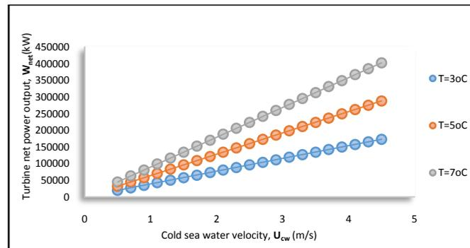
**Figure 8:** Variation of Turbine Net Power Output,  $W_{net}$  with cold Sea water velocity,  $U_{cw}$  at Different Temperatures.
