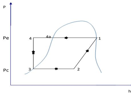
Figure 4: Pressure –Enthalpy Diagram of the Cycle.
