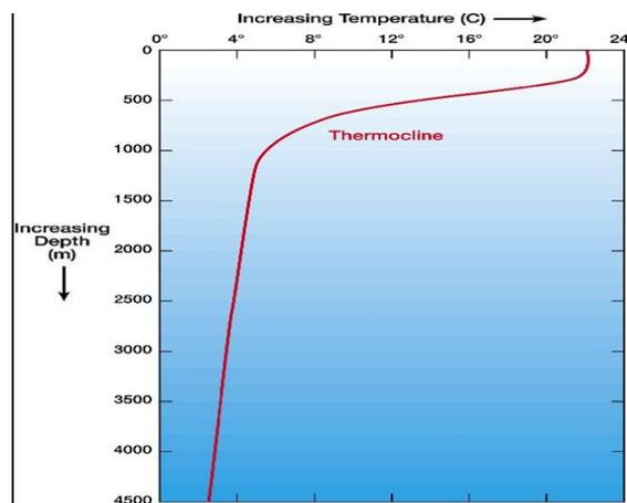
Figure 2: Temperature- Depth Ocean Water Profile [10].
