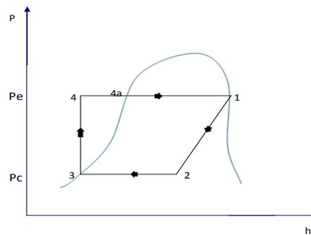
**Figure 4:** Cycle Pressure-Enthalpy (P-h) Diagram.
