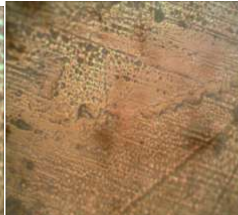
Figure 15: Microstructural view of 70% VLDPE- 30%PTA
