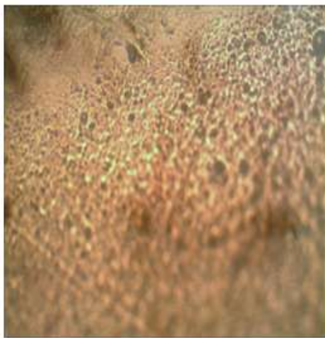
Figure 12: Microstructural view of 100% VLDPE- 0%PTA
