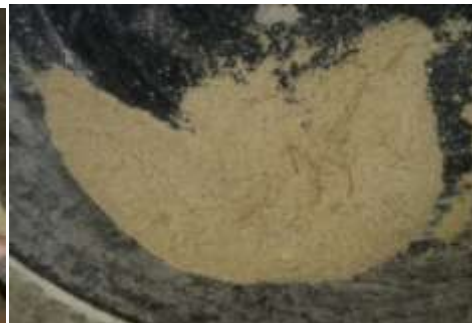
Figure 4: Grounded palm trunk (palm trunk ash).
