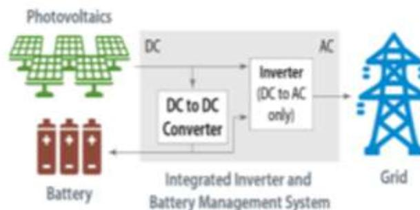
**Figure 6.0:** DC Tightly Coupled PV Plus Storage Systems.
