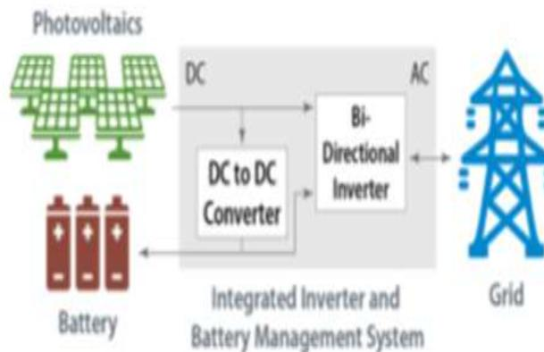
**Figure 5.0:** DC-Coupled PV Plus Storage Systems
