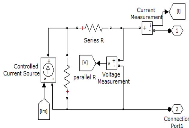
Figure 10.0: Solar PV Model in MATLAB/Simulink (Khamis et al, 2011).
