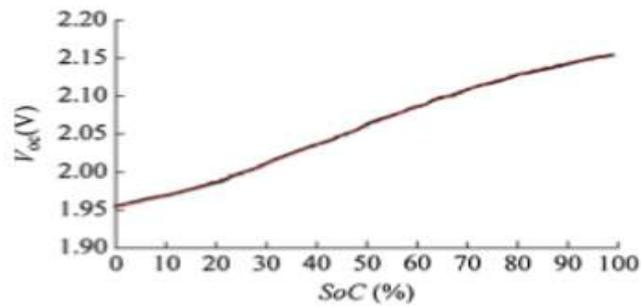
Figure 2.0: Open-Circuit Voltage characteristics
