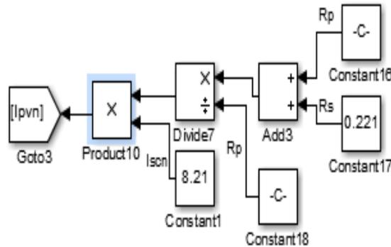
Fig 15.0: Building Block of Solar PV Model in MATLAB/Simulink
