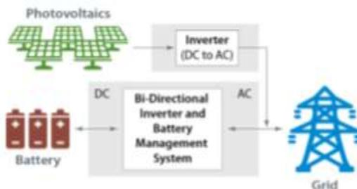
Figure 4.0: AC-coupled PV plus storage System
