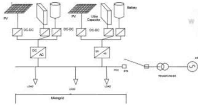
Figure 7.0 Microgrid Topology
