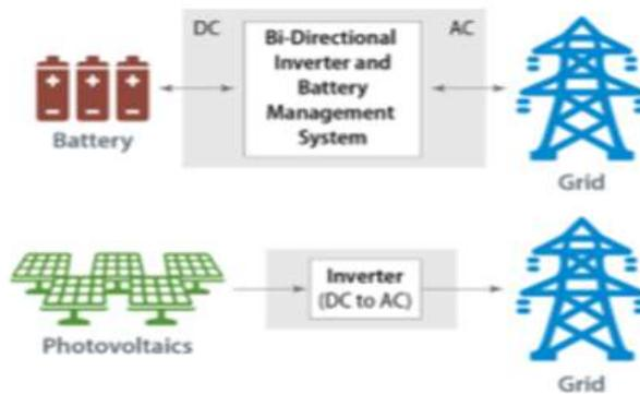
Figure 3.0: Independent PV and Storage Systems
