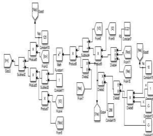
Figure 11.0: Complete Solar PV Model in MATLAB /Simulink Platform
