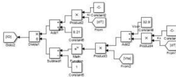
Fig 13.0: Building Block of Solar PV Model in MATLAB/Simulink
