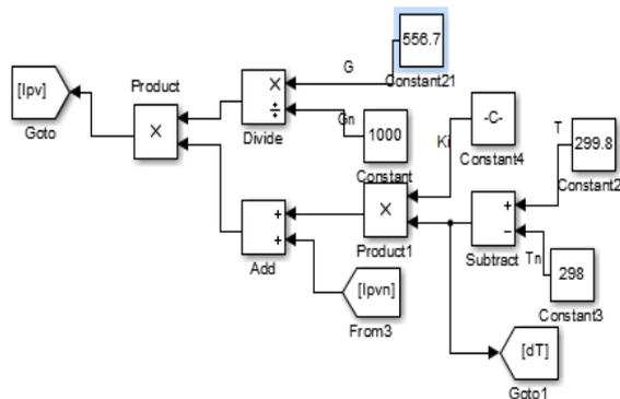
Fig 14.0: Building Block of Solar PV Model in MATLAB/Simulink
