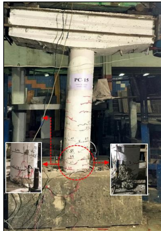
(e) Specimen PC-15 at Failure
