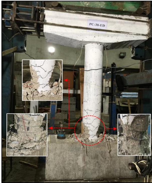
(b) Specimen PC-30-ED at Failure
