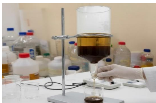
Fig. 3. PKO Biodiesel Separation Process
