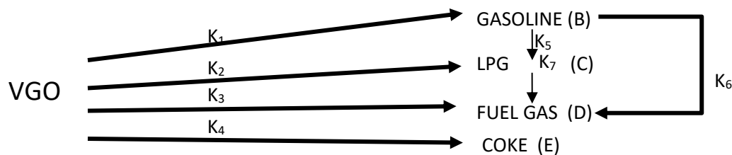
Figure 1: Five Lumps Reaction Scheme
