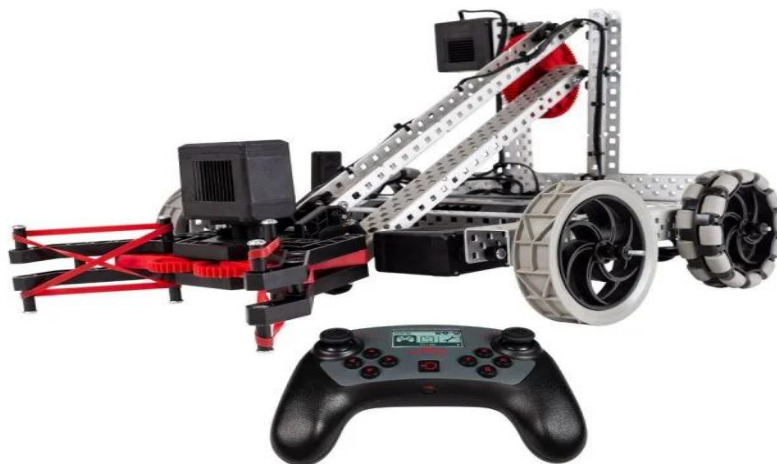
Figure 1 Example VEX V5 robot build (clawbot platform) with controller. The metal chassis and omnidirectional wheels enable robust mobile base.
