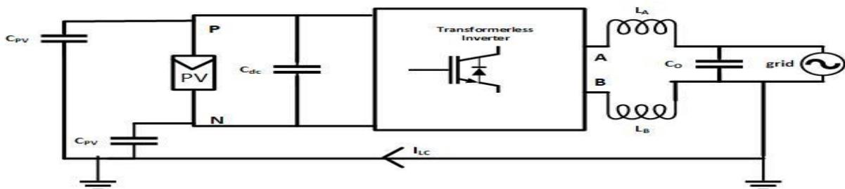
Figure 1: Leakage current flowing path in transformerless inverter
