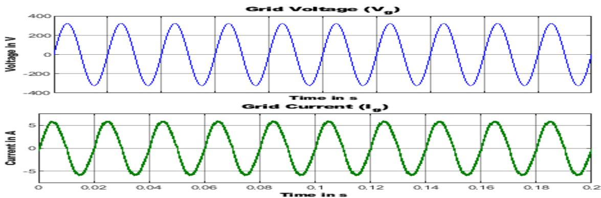
Figure 23: Output static performance of OH5 topology for closed loop with 1KW fixed active power
