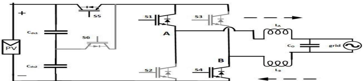
Figure 9: Positive half cycle active mode of OH5 topology
