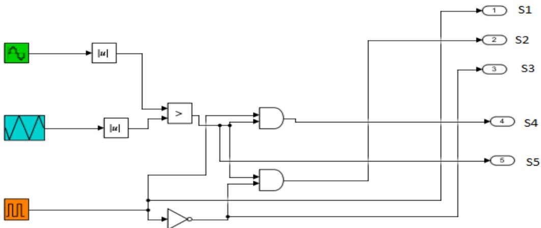
Figure 13: Pulse generation process of H5 topology
