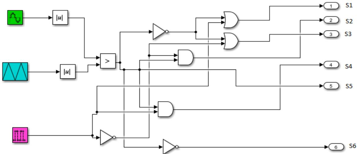
Figure 14: Pulse generation process of OH5 topology
