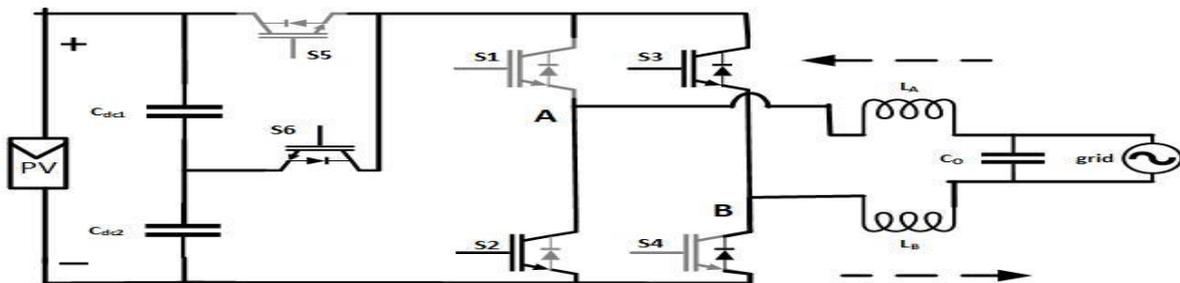
Figure 12: Negative half cycle freewheeling mode of OH5 topology
