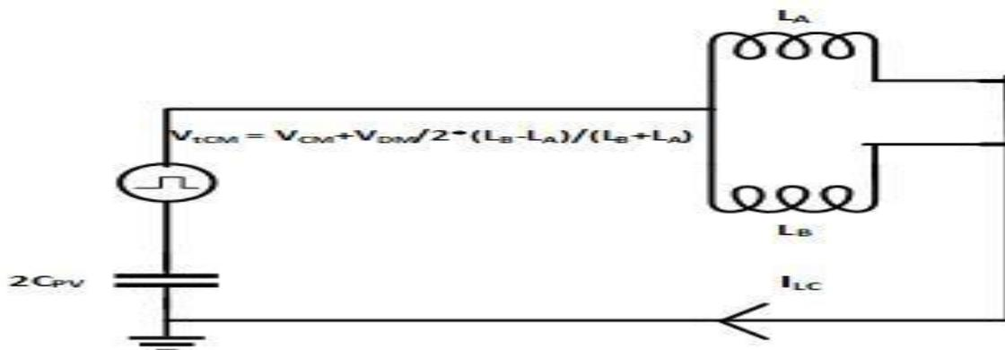
Figure 2: Final model of leakage current flowing path of transformerless inverter
