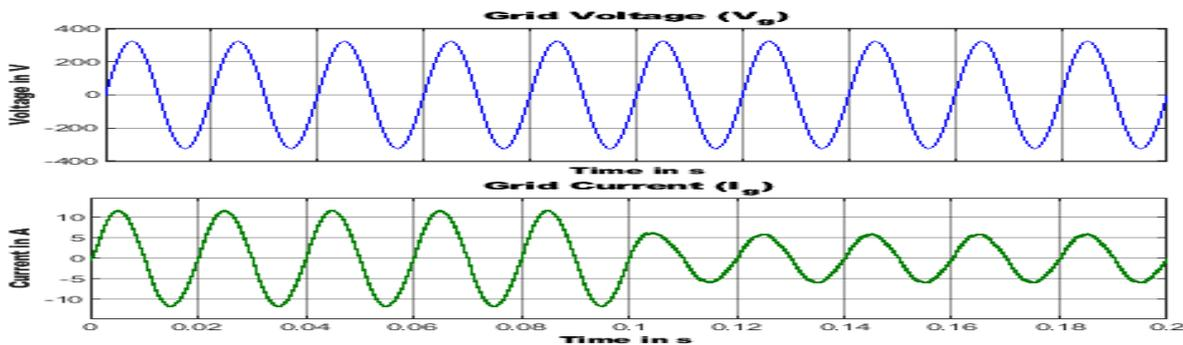
Figure 24: Output dynamic performance of OH5 topology for closed loop from 2KW to 1KW active power switching
