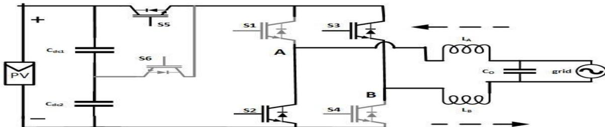
Figure 11: Negative half cycle active mode of OH5 topology
