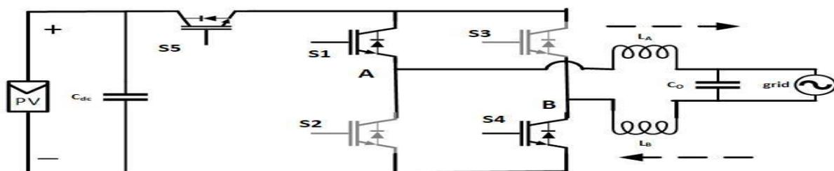
Figure 5: Positive half cycle active mode of H5 topology
