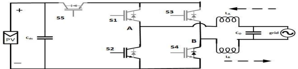
Figure 8: Negative half cycle freewheeling mode of H5 topology
