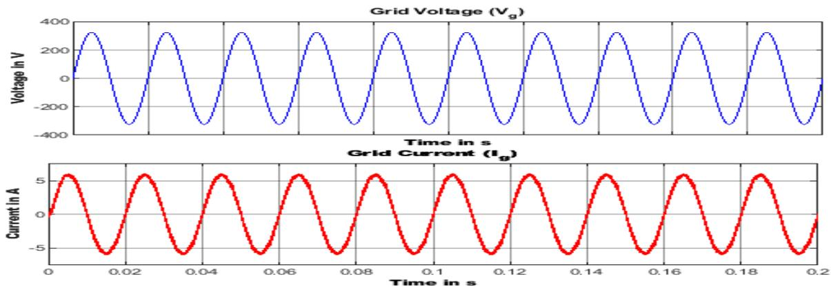
Figure 20: Output static performance of H5 topology for closed loop with 1KW fixed active power
