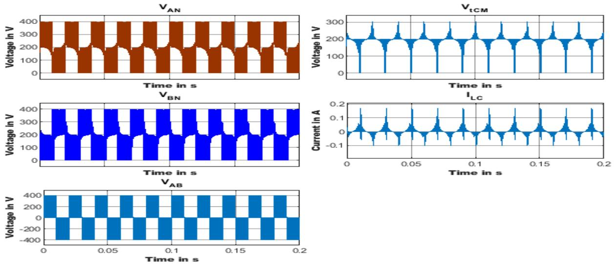
Figure 19: Common mode behavior of H5 topology for closed loop
