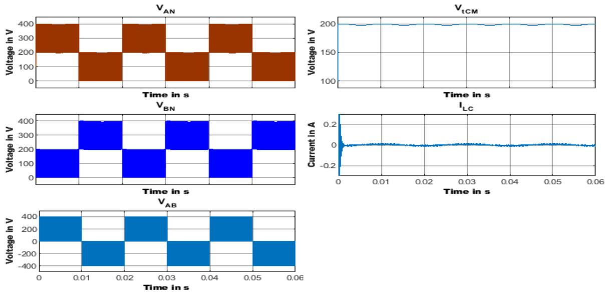
Figure 17: Common mode behavior of OH5 topology for open loop
