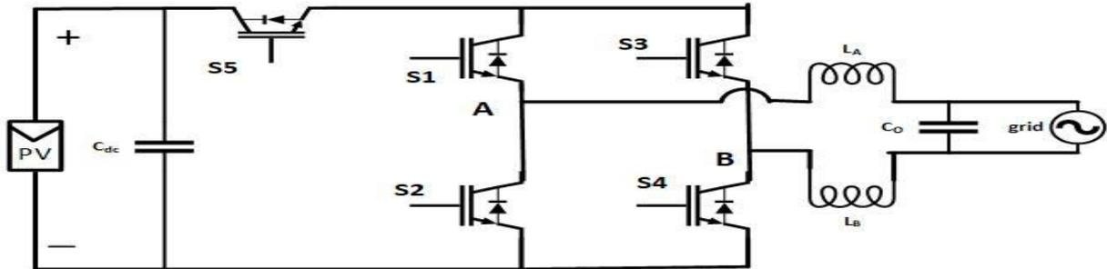
Figure 3: Circuit structure of H5 topology
