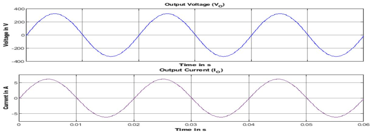
Figure 16: Output voltage and output current of H5 topology for open loop
