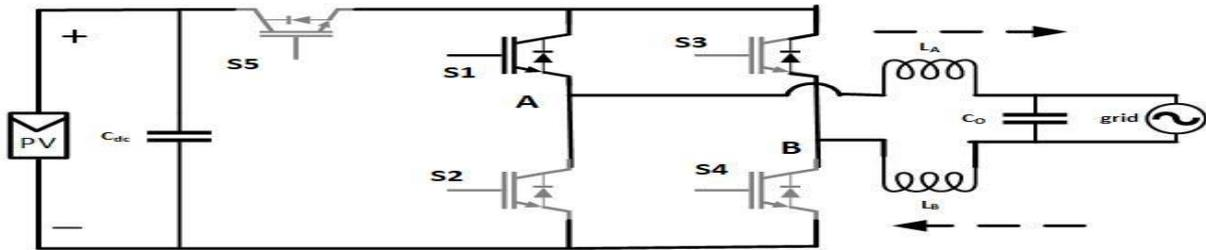
Figure 6: Positive half cycle freewheeling mode of H5 topology
