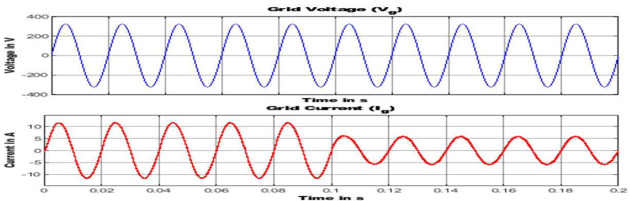
Figure 21: Output dynamic performance of H5 topology for closed loop from 2KW to 1KW active power switching
