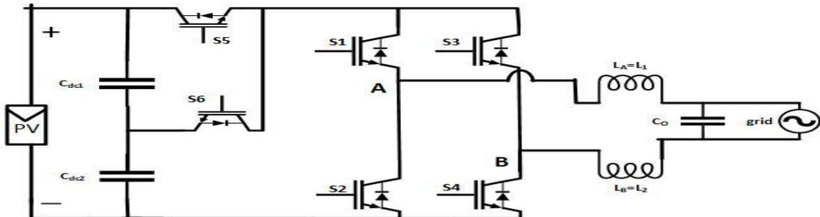
Figure 4: Circuit structure of OH5 topology
