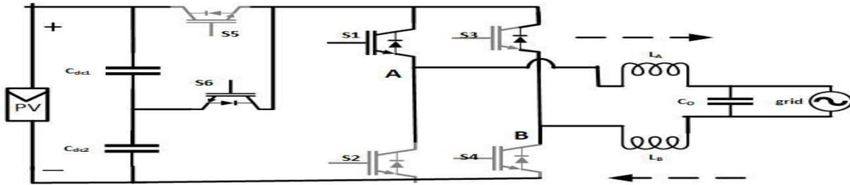
Figure 10: Positive half cycle freewheeling mode of OH5 topology
