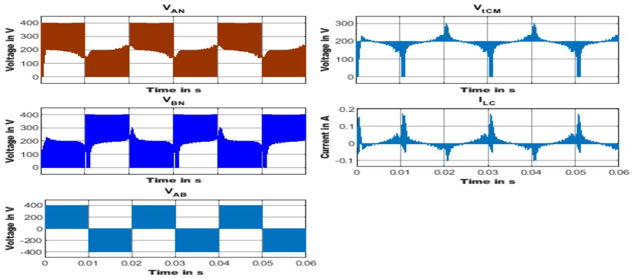
Figure 15: Common mode behavior of H5 topology for open loop
