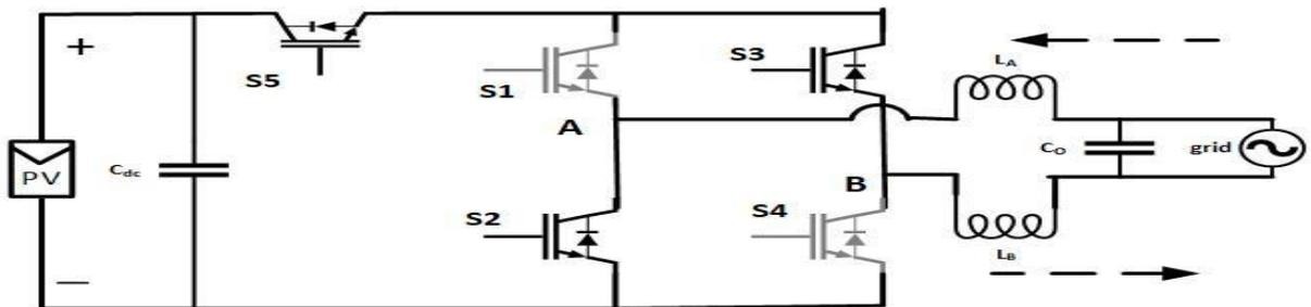
Figure 7: Negative half cycle active mode of H5 topology
