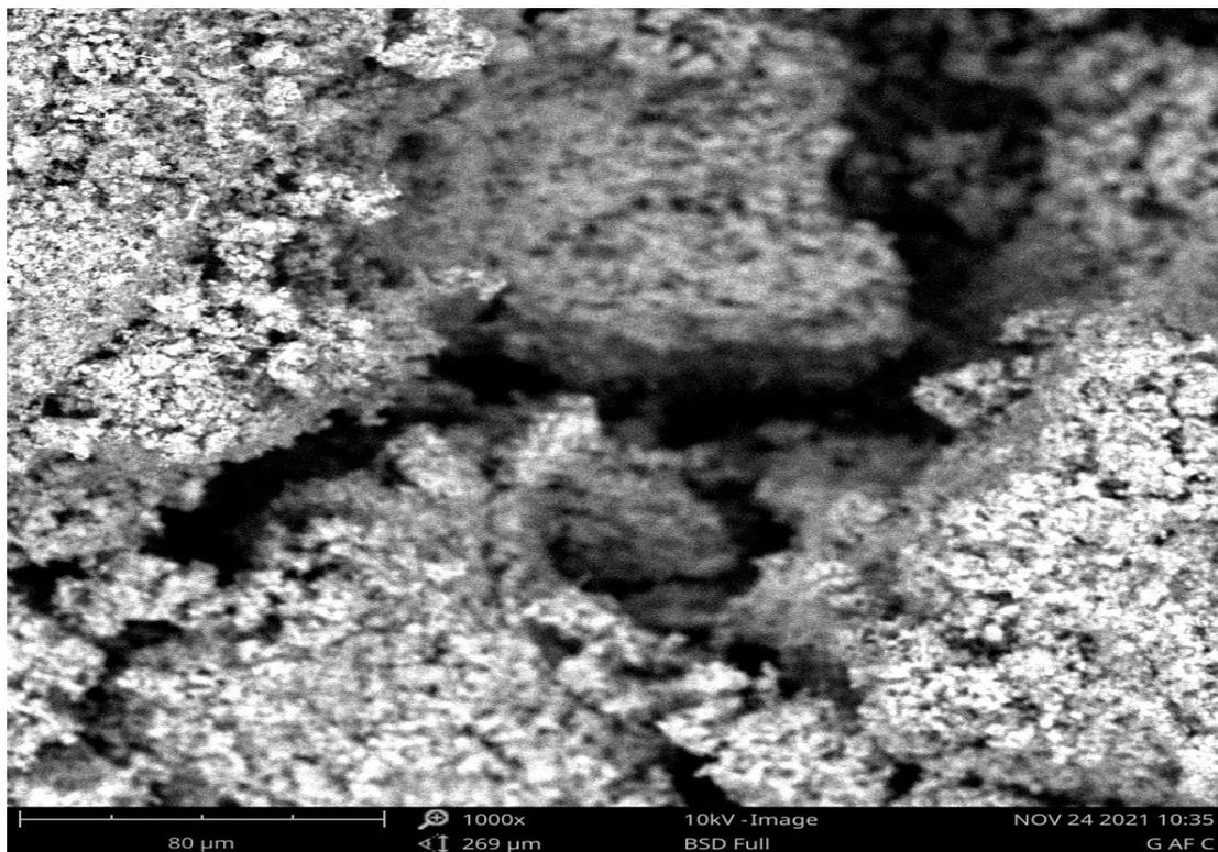
Figure 8: SEM of Gelling Agent from Corncob (Na-CMC)
