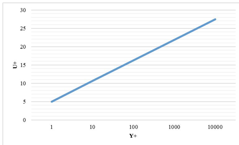
**Graph(4): shows the velocity profile of a turbulent boundary layer**
