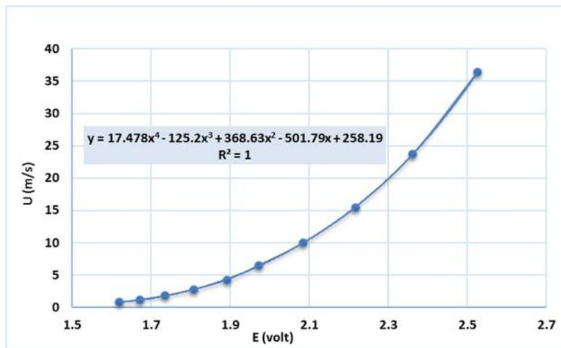
**Graph (1): shows A typical single wire calibration curve**
