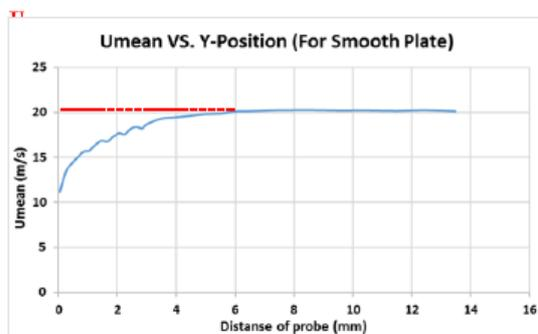
**Graph (2):shows  $U_{mean}$  VS. Y-position for smooth plat for riblet plat**
