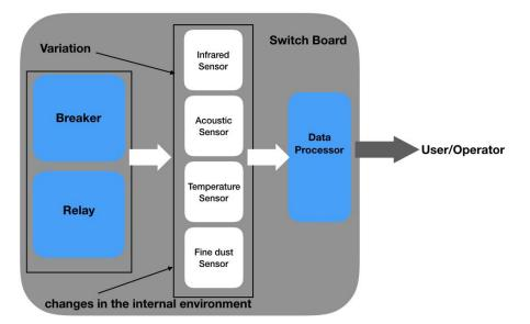
Pic. 2 Work Process in Smart Switch Board
