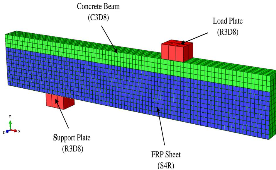
Fig. 5. Quarter of strengthened RC beam.
