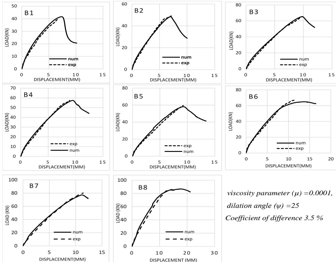
Fig. 8. Experimental versus Numerical ultimate load-displacement curves.
