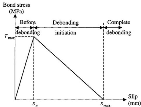
Fig. 4. Bilinear bond-slip model [11]
