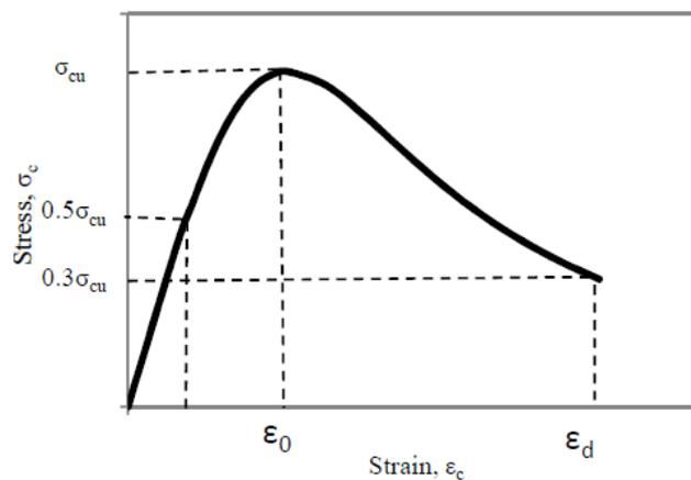
Fig.1. Concrete Compressive behavior [16]
