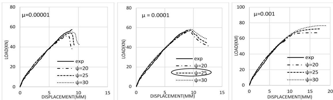
Fig. 7. Ultimate load-displacement Attempts for Specimen b4
