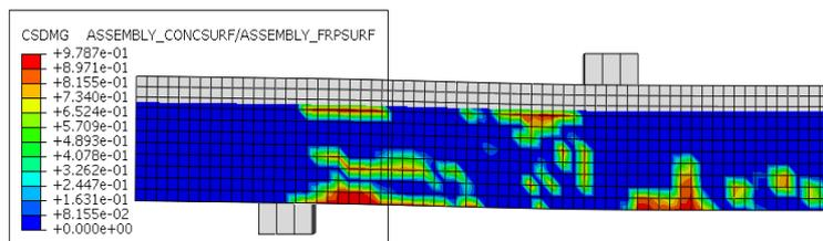
(f) ABAQUS Output, FRP debonding failure
