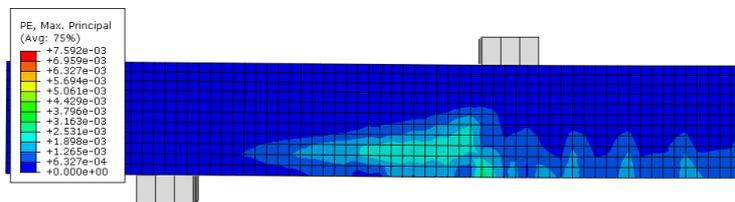
(c) ABAQUS Output, Crack pattern of RC beam
