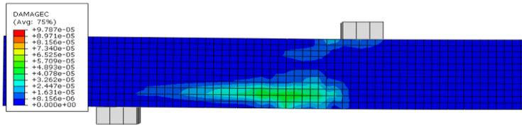
(b) ABAQUS Output, Compression damage of RC beam
